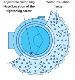
the floor drain or the build-up ring as well as the lip seal in the upper rim. Merika water insulation flange is installed to its place and the drain seal remains in its groove. The water insulation flange is clamped in its place to the drain according to the installation instructions of the water insulation flange. Remove any air bubbles with a trowel.
