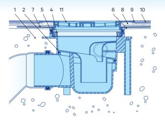
Installing a MERIKA® water insulation flange with a square cover in the floor drain with a build-up ring in a thermally insulated concrete floor
